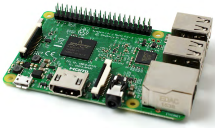
Figura 2.17: Raspberry Pi 3 Model B. Figura extraída de ( Upton e Halfacree, 2014 )
